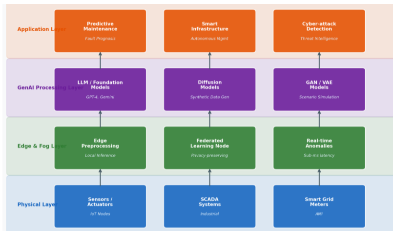
Figure 1. Layered Architecture of Generative AI in Cyber-Physical Systems. The four-tier model spans physical sensing, edge preprocessing, cloud-based generative modeling, and intelligent application services. Arrows denote bidirectional data flows. Adapted from the architectural framework proposed by Deng et al. [6].
